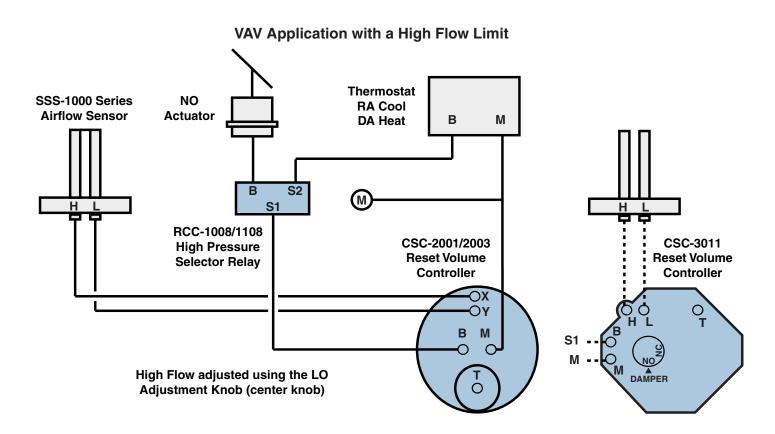
NOTE: On the CSC-3011, ensure the Damper Action Selection Dial is set properly (Normally Open in these examples).
