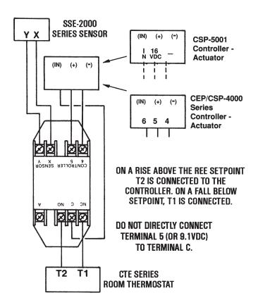
NOTE: **Terminal A** is an optional **auxiliary flow** limit trigger signal (usually connected to Terminal A on a CTE-1004, CTE-5104, or REE-1012). When the relay module senses heating mode, terminal A goes high (around 6.8 VDC with a 9.1 VDC supply or 13.8 VDC with a 16 VDC supply). This terminal can also be used to daisy chain more than one REE-1005 together by wiring Terminal "A" to Terminal "Y" on the next relay.
