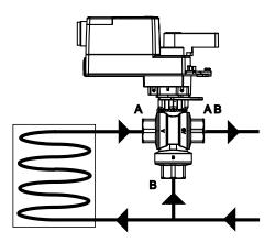
DIVERTING Flow Action: Full CCW = Port AB to A Full CW = Port AB to B
