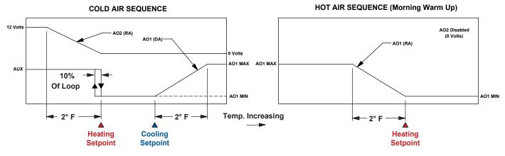
SEQUENCE # 2: SINGLE DUCT COOLING WITH REHEAT AND AUXILIARY FLOW
