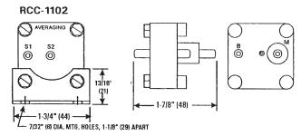
Main air is Port M and output is Port B. Inputs to be averaged are applied to S1 and S2.
