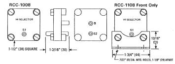
No adjustments need to be made. The design allows for positive switching between signals, and the non-transmitted signal is internally blocked. The signals applied to Ports S1 and S2 must come from "relieving" type devices. Do NOT supply from NO or NC ports of diverting relays or solenoid air valves.
