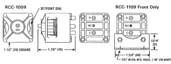
The setpoint dial can be rotated within the body to adjust the switching point. One turn yields approximately 6 psi change in the switching point. Each unit is factory-set to switch between 18 and 23 psi, which allows it to match most two-pressure main air systems. This device is not "snap-acting" (it must receive a positive pressure change at its signal port to switch).
