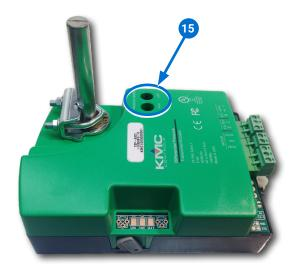
2. Connect the high pressure tube from the pressure flow sensor to the **HIGH** 16 port on the controller.
