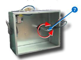
**NOTE:** The drive hub and V-clamp will be rotated in the same direction in Step 3.
