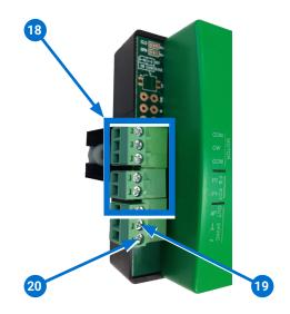
NOTE: Terminals P1 and P2 provide feedback on damper position with a 10K ohm (1/3 watt) potentiometer (10K ohms full CW and 0 ohms CCW). They are not polarity sensitive. Connect them to controller inputs if desired (UI6 and GND on a BAC-9000 series controller).
