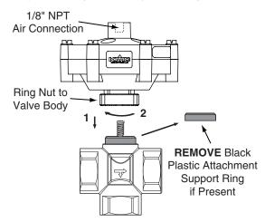
Mounting Actuator on Valve Body
