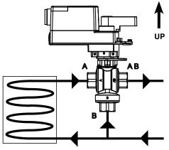
MIXING Flow Action: Full CCW = Port A to AB Full CW = Port B to AB
