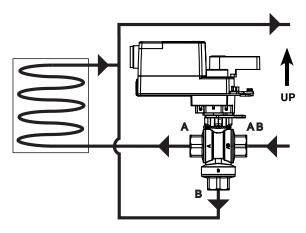
DIVERTING Flow Action: Full CCW = Port AB to A Full CW = Port AB to B
