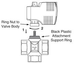
Mounting Actuator on Valve Body
