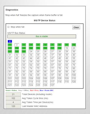
Offload MS/TP and routing from integration engine or supervisory controller.
