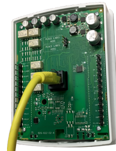
Illustration 9—Ethernet Network Connection ("E" Models)
