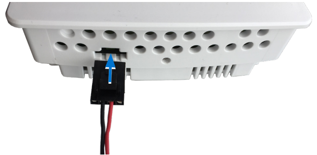
Illustration 14—MS/TP (EIA-485) Data Port
