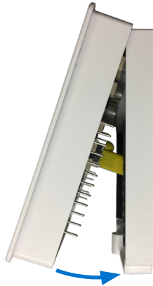
Illustration 7—Reinstalling the Cover on the Backplate
