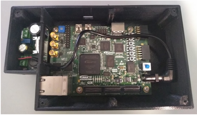
Fig. 6. DOME Sentry prototype based on MAX 10 (shown with cover removed)
