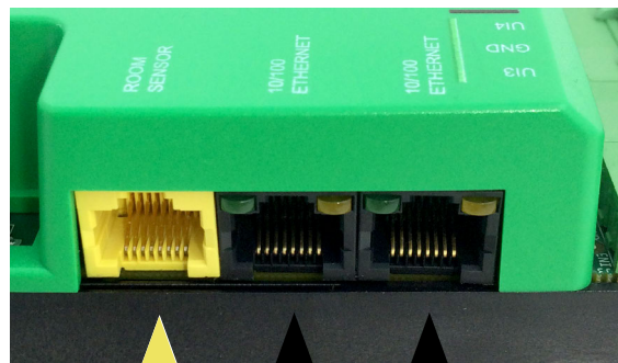
Illustration: Inputs and Ports (Early BAC-9001CE)
