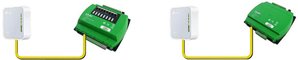
BACnet over IP Controllers (Wireless, One-to-One)
