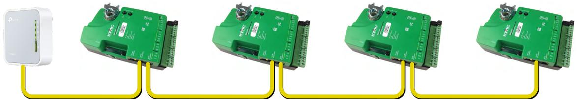
**BACnet over IP Network Controllers (Wireless, One-to-Many)**
