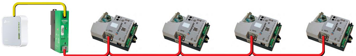
**BAC-5051E BACnet Router and MS/TP Network Controllers (Wireless, One-to-Many)**
