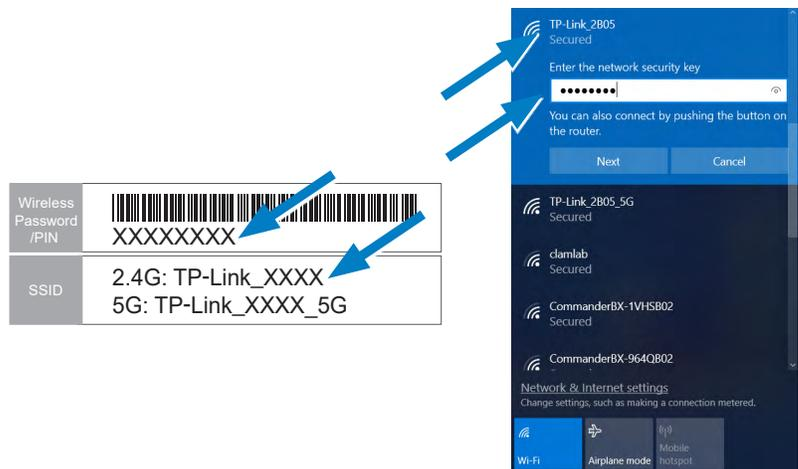
**NOTE:** Your router's default SSID (network name) and password are printed on a label on the back of the router.
