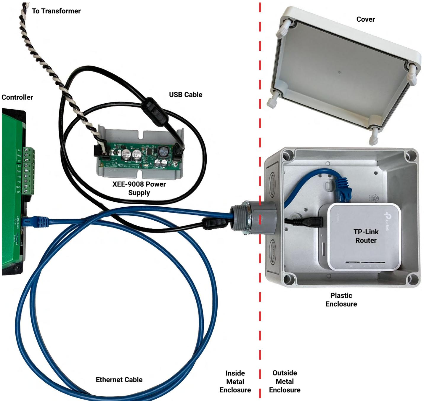
1. Loosen the four screws on the supplied plastic enclosure and remove the cover.
