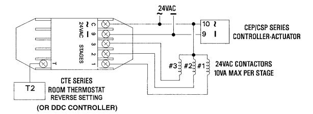
NOTE: Triac stages 1 through 3 are for 24 VAC loads only. This "C" terminal does NOT denote Common/Neutral. "C" is the phase side of the 24 VAC (and the phase side is where the three contactors are connected in "common"). "9" is the neutral side.
