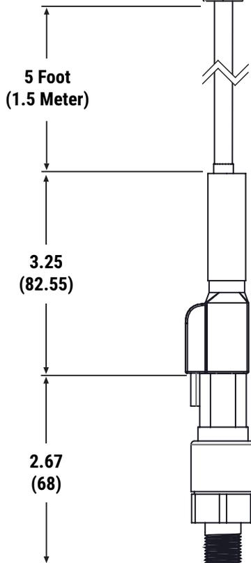
**NOTE:** Mount the transmitter on a vertical surface within 5 feet (1.5 meters) of the pressure port to be measured. Use #10 screws (not supplied) through the two integrated mounting holes. The remote sensor cable connection should be located on the bottom of the enclosure. Ensure there is enough space around the unit to make the electrical connections. Avoid locations with severe vibrations or excessive moisture.
