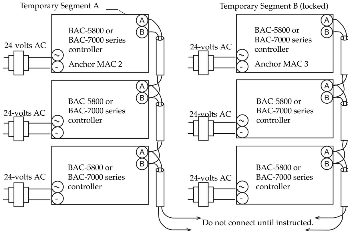
**Illustration 2-1 Figure 2: Combining locked and assigned network segments**
