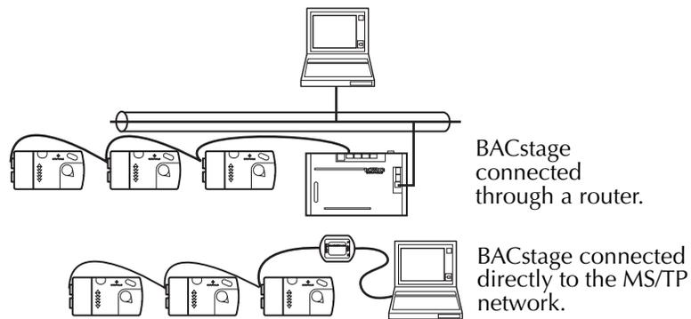
**Illustration 4-1 BACstage connections to an MS/TP network**
