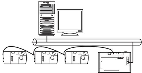
TotalControl connects to an MS/TP network through a router.
