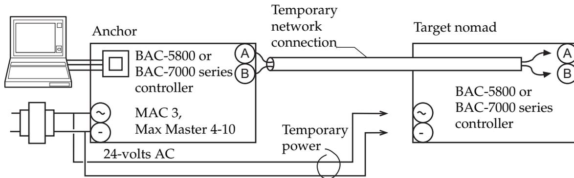
**Illustration 3-1** Bench setup for programming nomad controllers
