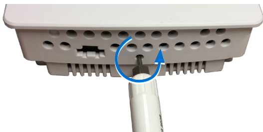
Illustration 8—Locking the Cover on the Backplate
