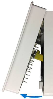
Illustration 4—Removing the Cover from the Backplate
