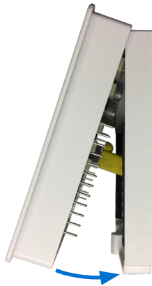
Illustration 7—Reinstalling the Cover on the Backplate
