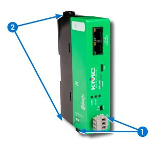
**NOTE:** Pull out each DIN Latch mounting tab one click to be 6 inches on center for mounting.
