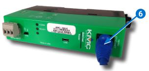
**NOTE:** The Ethernet cable should be a CAT 5 or better and a maximum of 328 feet (100 meters) between devices.
