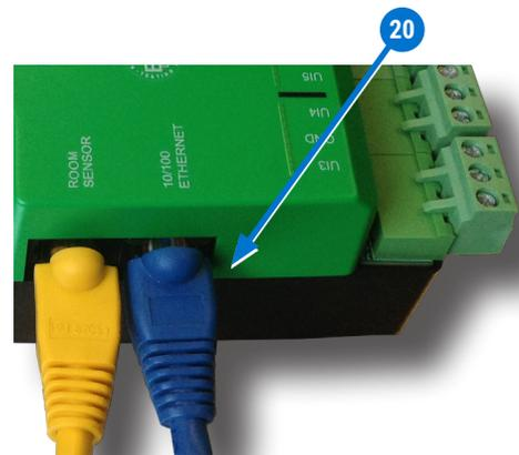
**NOTE:** Also on the newer models, the Room Sensor port is **yellow 22** instead of black to help differentiate it from the black Ethernet ports.
