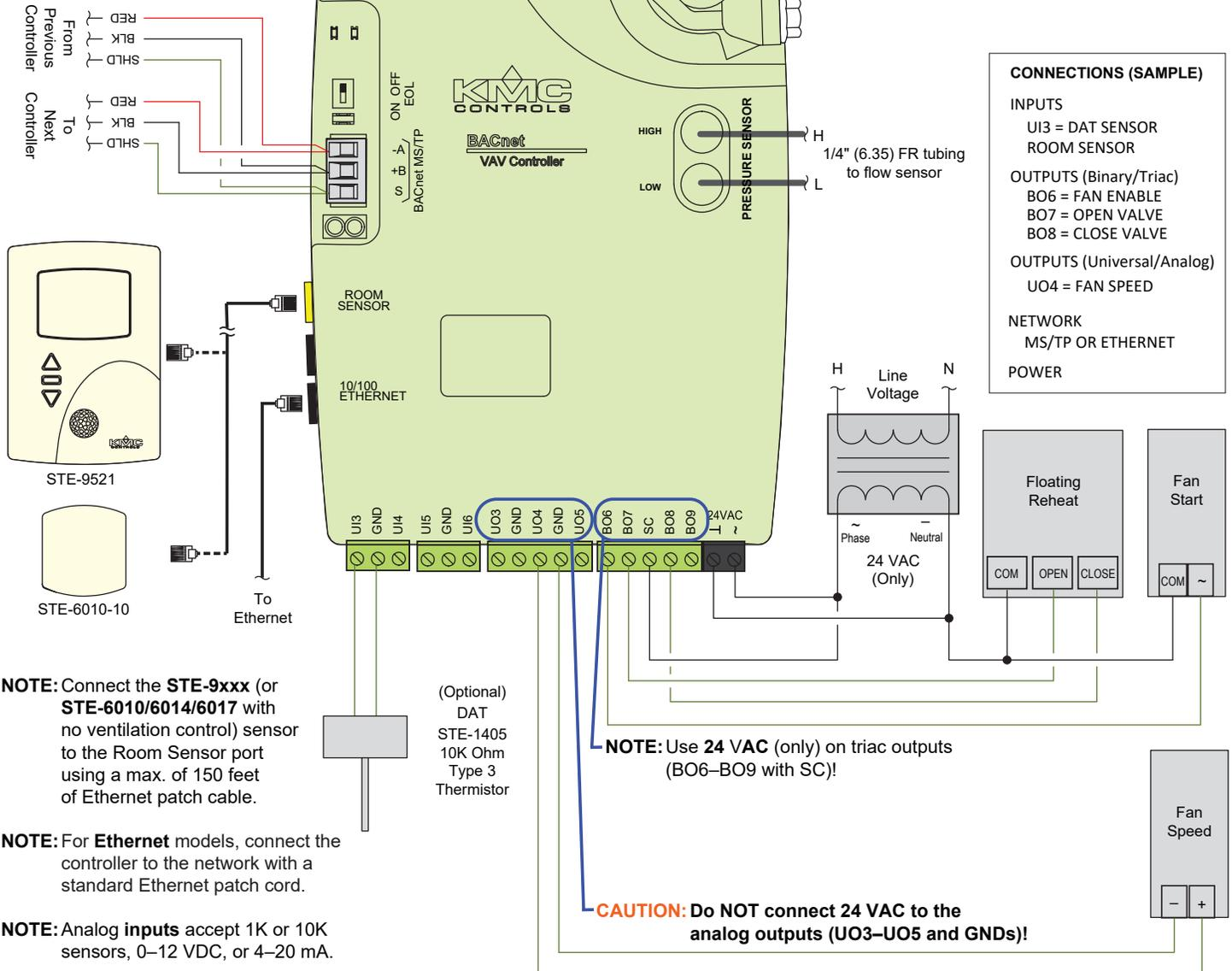
**NOTE:** Connect the **STE-9xxx** (or **STE-6010/6014/6017** with no ventilation control) sensor to the Room Sensor port using a max. of 150 feet of Ethernet patch cable.
