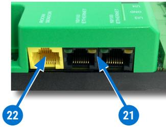
**NOTE:** The Ethernet patch cable should be T568B Category 5 (or better) and a maximum of 328 feet (100 meters) between devices.
