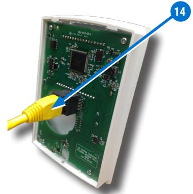
**NOTE:** The Ethernet patch cable should be a maximum of 150 feet (45 meters).
