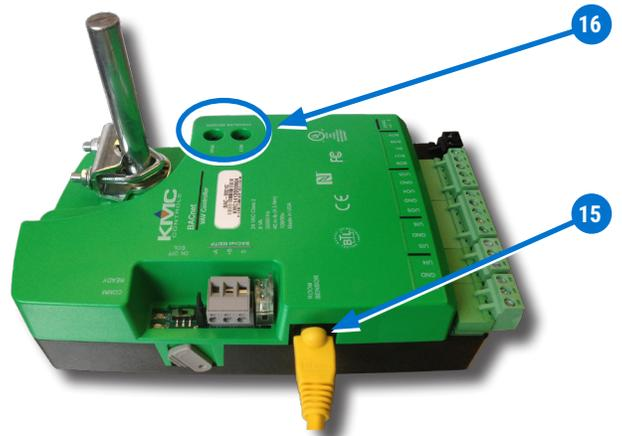
**NOTE:** Auxiliary VAV equipment such as fans, heaters, reheat valves, and discharge air temperature sensors can be connected to the controller.
