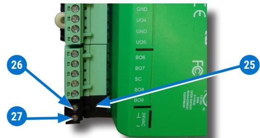
**NOTE:** Connect only one controller to each transformer with 12–24 AWG copper wire.
