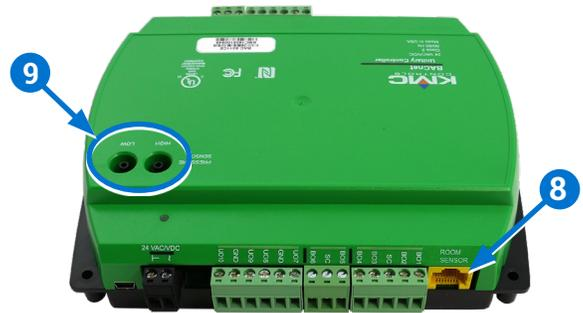
2. Wire any additional sensors to the **green (input) terminal block** **10**. See **Sample (BAC-9311) Wiring on page 7**.
