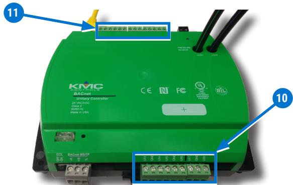
3. Wire additional equipment (such as fans, heaters, dampers, and valves) to the **green (output) terminal block** **11**. See **Sample (BAC-9311) Wiring on page 7**.
