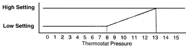
**Reverse Acting GRAY units (CSC-2002/2004/2008/2010/2018)** are designed for normally closed dampers with reverse-acting thermostats for cooling and direct-acting thermostats for heating.
