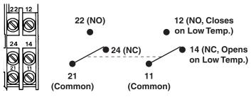
(Connections Shown in Above-Setpoint, NC, Unactuated Position)
