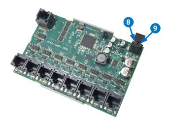
NOTE: Connect only **one** module or controller to a 24 VAC, Class-2 transformer with 12– 24 AWG copper wire. (See **Transformers**, **120 to 24 VAC on page 5**.)
