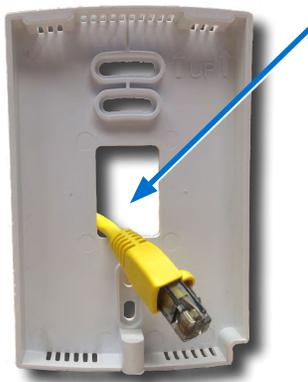
**NOTE:** The Ethernet patch cable should be a maximum of 150 feet (45 meters).
