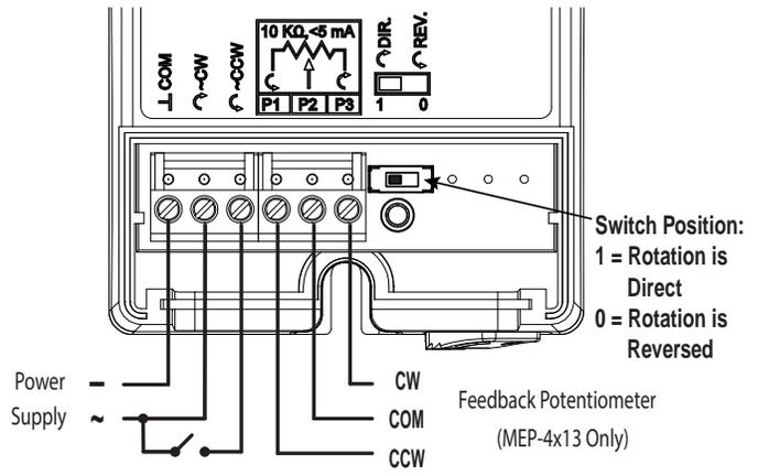
Contact Position: Open = CW Rotation, Closed = CCW Rotation
