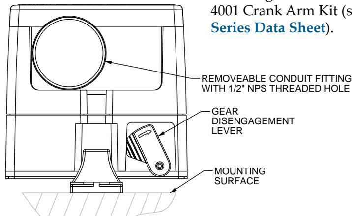
1. Ensure the damper can move freely through its entire range of motion, and fix any binding before installing the actuator. Turn the damper blade to its fully closed position.
