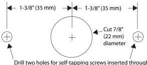
Drill two holes for self-tapping screws inserted through the pickup tubes' 3/16" (5 mm) mounting holes.
