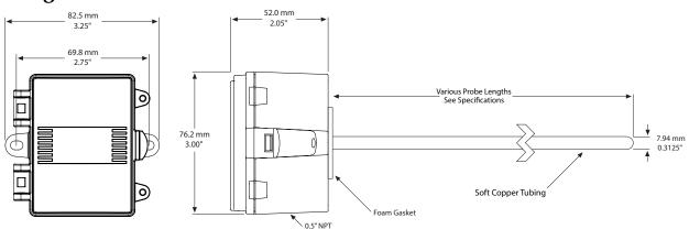
The averaging temperature sensor incorporates several discrete sensors encapsulated at equal distances across the length of the copper tubing probe. The complete assembly acts as a single sensor to monitor the average temperature in a duct. (Averaging elements are not recommended for high humidity applications.)
