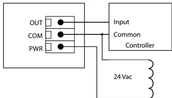
24 Vdc Power Supply, 0-10 Vdc Output
