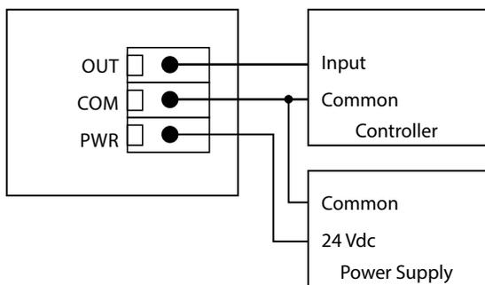
24 Vdc Power Supply, 4-20 mA Output
