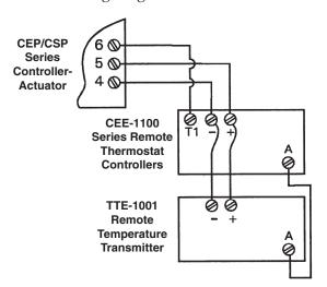
NOTE: This TTE-1001/CEE-11xx configuration can be used in place of an applicable CTE-11xx room thermostat.
