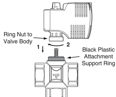
Mounting Actuator on Valve Body
