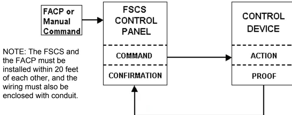
**Figure 3: Block Diagram of a Smoke Control System**
