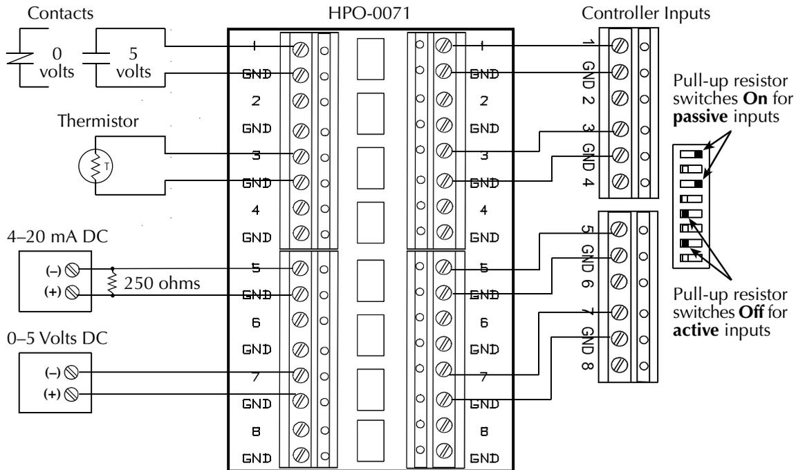
**Figure 9: Typical Input Configurations (with HPO-0071 Transient Suppressor Board)**
