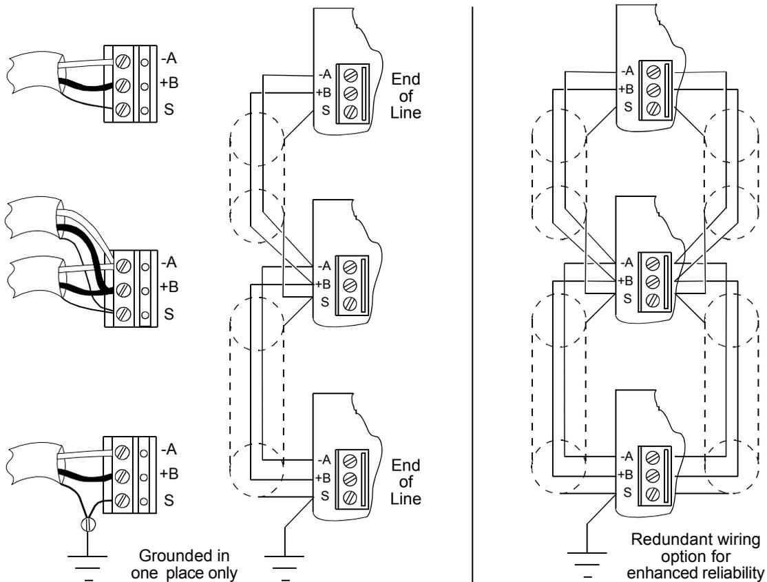
**Figure 8: EIA-485 Network Wiring Details and Redundant Option**
