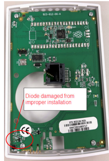
Exposed printed circuit board showing area of damage
